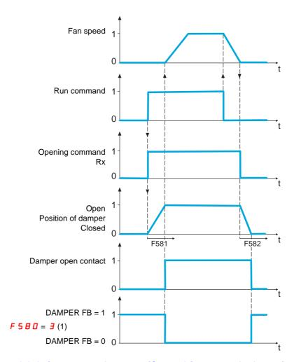
(1) [Com channel choice] F B D 7 must be set to I [Open style] to manage the damper feedback on BACnet network. DAMPER FB can only be active when [Damper fdb type] F 5 B D is set to J [Com. LIL set] or 4 [Com. LIH set].
